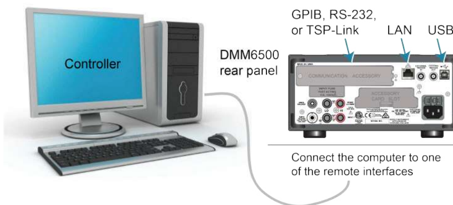
Figure 15: DMM6500 remote interface connections
