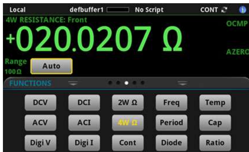
Figure 37: 4-wire resistance test results
