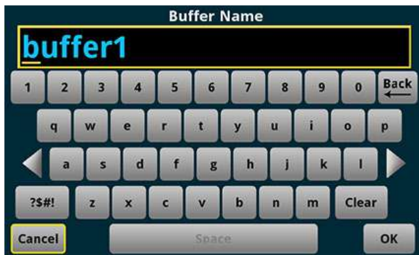
Figure 3: DMM6500 front-panel keyboard for information entry
