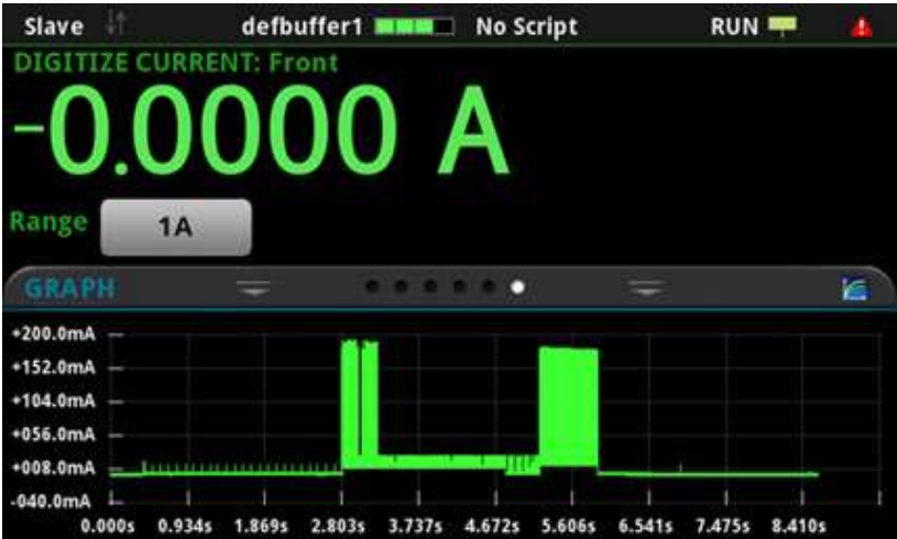
Figure 48: Subordinate node current waveform
