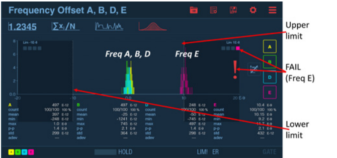
The Frequency distribution view reveals the spread (stability) of the oscillators
