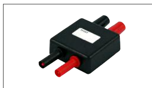
910007200: 0.1 ohm shunt, 1%, 1A max
