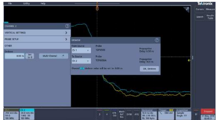
Figure 6. Nominal Correction of Timing Skew between Voltage and Current Probes.
