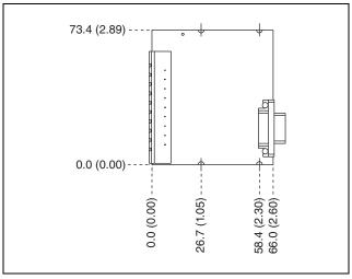
Figure 1. NI 9265E Dimensions in Millimeters (Inches)
