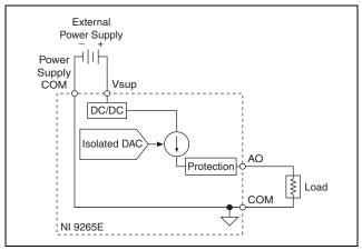
Figure 3. Connecting a Load to the NI 9265E
