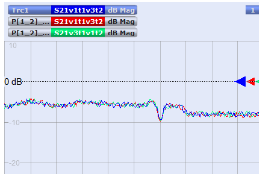
Figure 5-17: Multiple traces due to multiple paths
