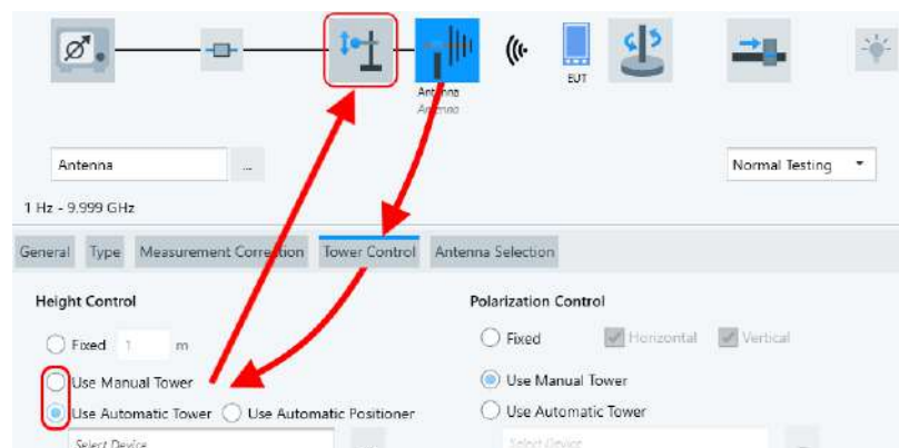
Figure 4-140: Integrating an antenna tower into the Electric Field Strength hardware setup
