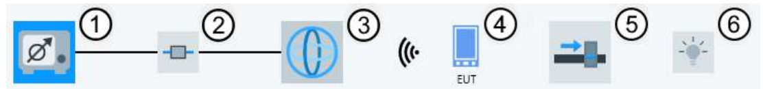
Figure 4-142: EMI radiated hardware setup diagram Magnetic Field Strength (Triple Loop Antenna)
