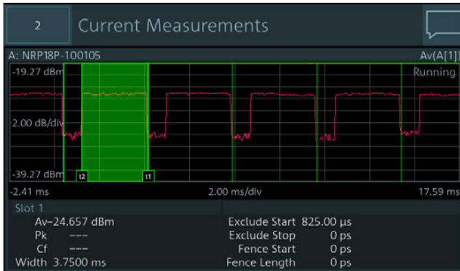
Timeslot measurement of a Bluetooth® signal with exclude start time
