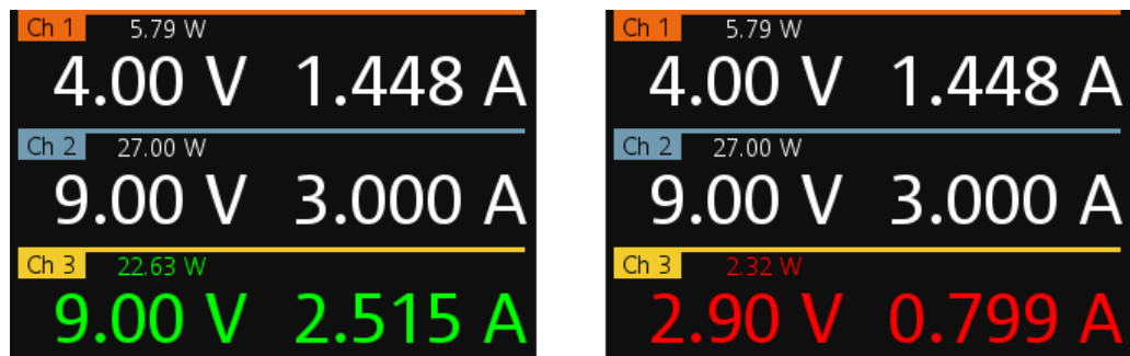
Figure 6-3: Output of Ch 3 in CV and CC mode
