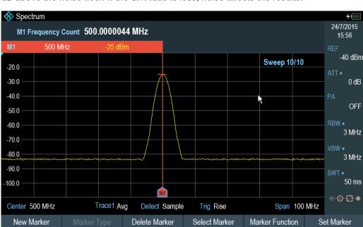
The frequency counter only gives accurate readings for sine signals that are at least 20 dB above the noise floor. If the S/N ratio is less, noise affects the results.
