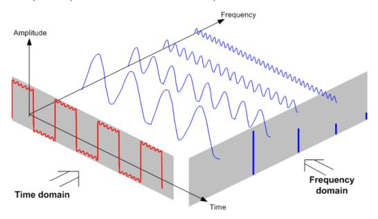
Figure 17-1: Visualization of time domain and frequency domain
