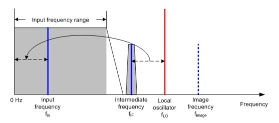
The first local oscillator is tuned with a sawtooth which simultaneously acts as the x deflection voltage for the display. In practice, synthesizer technology is used to generate the frequency of the first local oscillator and for a digital display.
