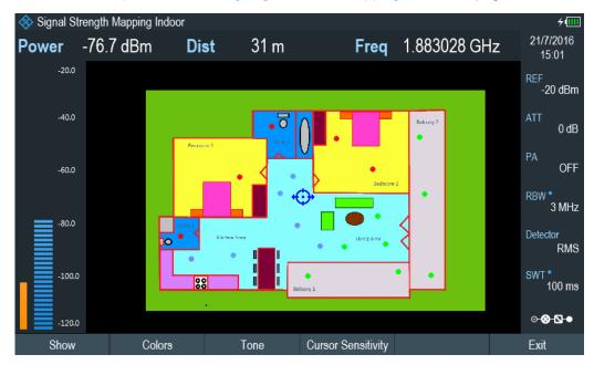
Figure 11-8: Tags on indoor mapping
