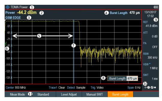
Figure 6-3: Screen layout for TDMA power measurements
