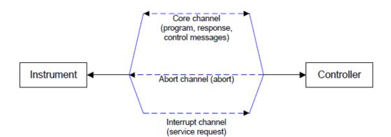
Figure 14-2: VXI-11 channels between instrument and controller
