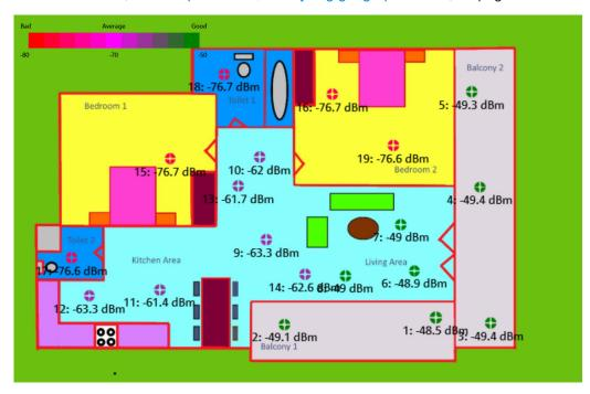
Figure 11-10: Indoor mapping with signal strength and indices displayed.
