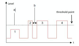
Figure 10-5: Burst signal conditions
