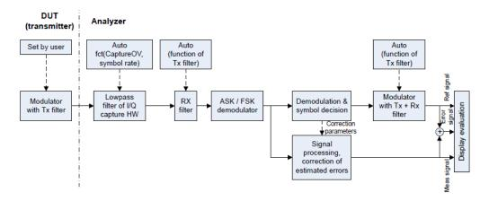
Figure 10-4: Block diagram of measurement filter
