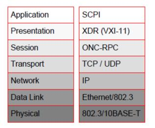
Figure 14-1: Example for LAN remote control based on the OSI reference model
