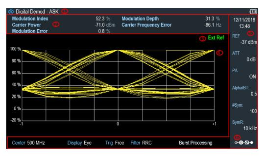
Figure 10-3: Eye diagram of an ASK modulated signal
