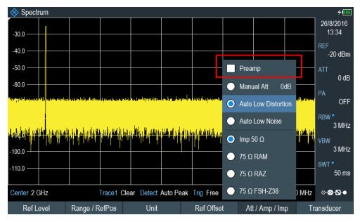
The magnitude of amplification depends on the reference level. This coupling to the reference level makes sure that the dynamic range is at an optimum.
