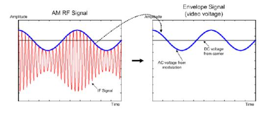
If the bandwidth of the video filter is less than the frequency of the AC component, it is suppressed depending on its maximum frequency. If the AM component should be displayed truly, the cutoff frequency of the filter has to be greater than the modulation frequency.
