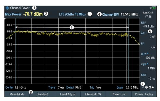
Figure 6-1: Screen layout for channel power measurements
