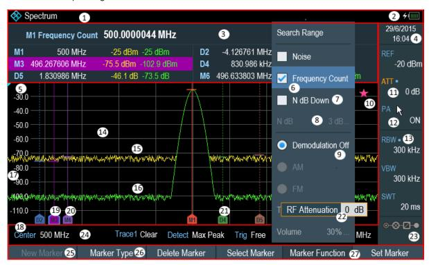
Figure 4-1: Screen layout and elements
