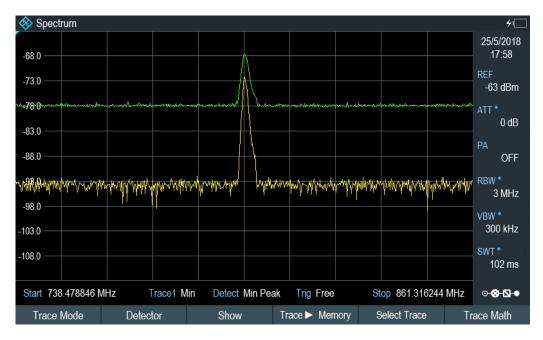
You can put both traces into the internal memory of the R&S Spectrum Rider and restore them later. Note that the memory trace 1 and memory trace 2 have a lighter tone color.
