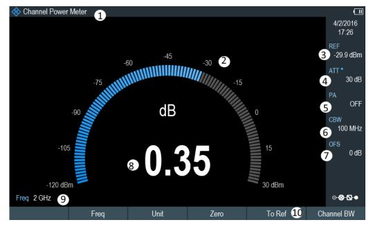
Figure 8-1: Channel power meter measurement
