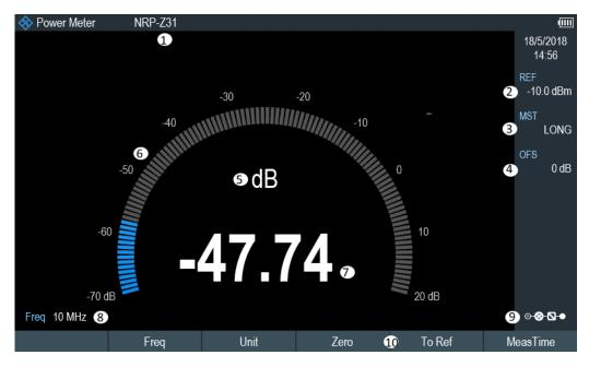
Figure 7-1: Screen layout of the power meter mode
