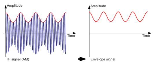
The video filter comes after the envelope detector. The filter is a lowpass with an adjustable cutoff frequency which limits the bandwidth of the video signal. It is particu-
