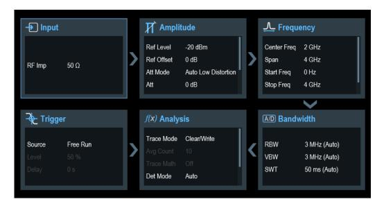
The "Configuration Overview" provides quick access and allows easy configuration on the parameters that affect the spectrum measurement from input to signal processing to output and signal analysis by stepping through each of the following dialog boxes:
