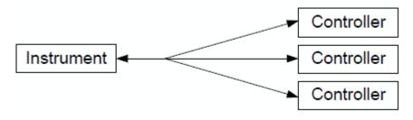
Figure 14-3: Remote control via LAN from several controllers
