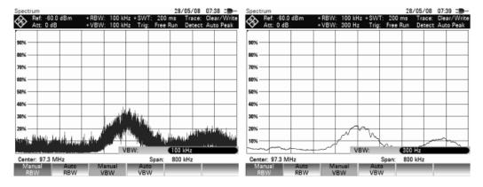
Limiting the video bandwidth smoothes the trace considerably. This makes it much easier to determine the level of the measured signal.
