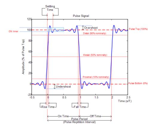
Figure 9-2: Graphical representation of pulse characteristic
