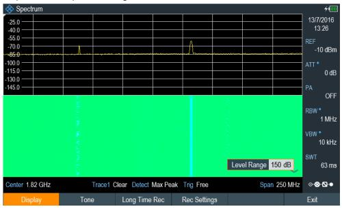
Example: If a spectrogram reference level is at -10 dBm, the signal parts with an amplitude of -10 dBm would be blue in the spectrogram. For signal parts with a very small amplitude, it is dark green. Everything in between is a shade of the colors between. As the colors are distributed over a very large range (150dBm), it is likely that you cannot distinguish details in the signal that you have measured.
