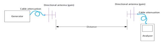
Figure 6-11: Test setup for EIRP measurement
