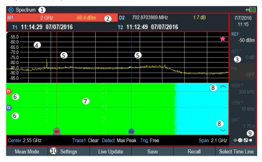
Figure 6-8: Screen layout for the spectrogram
