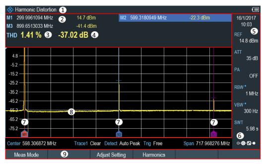
Figure 6-6: Screen layout for the harmonic distortion measurement
