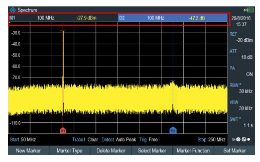
To measure the harmonic ratio, set the marker on the signal and a delta marker on the second harmonic.
