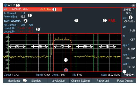
Figure 6-5: Screen layout for ACLR measurements
