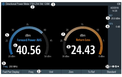
Figure 7-2: Screen layout of the directional power mode
