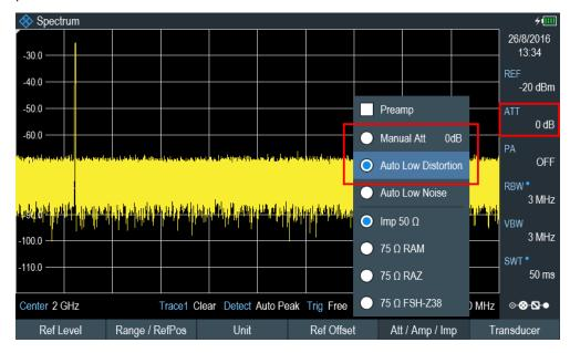
You can also set the attenuation manually. TheR&S Spectrum Rider provides attenuation in the range from 0 dB to 40 dB in 5 dB steps.
