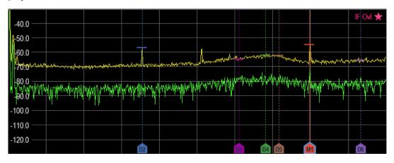
Device warning messages (e.g IF OvI) are displayed at the top right-hand corner of the window.
