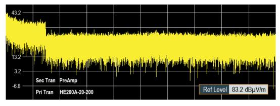
Figure 6-15: Transducer factors displayed
