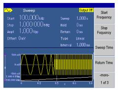
Frequency range from 1 µHz to 20 MHz, supports a wide range of amplifier and filter testing applications.
