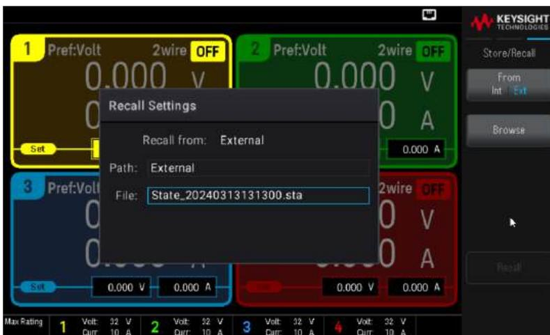
Source [Int](#) | [Ext](#) recalls the instrument state in a connected external USB flash drive.
