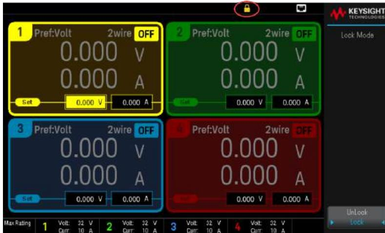
2. Select **Unlock** to unlock the front panel.
