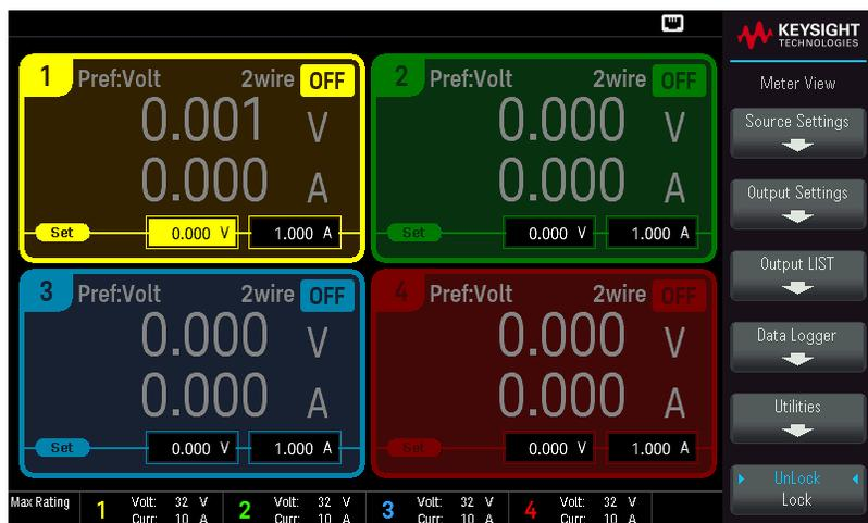
Lastly, you can press the **Source Settings** key to access the Source Settings window. Use the navigation keys to highlight the Voltage or Current fields. Then enter the voltage and current values with the numeric keys.
