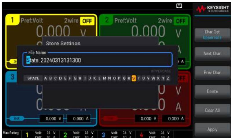
A virtual keyboard appears when you press certain softkey, for example **File Name**. This keyboard allows you to edit existing naming. Use the navigation keys, and the softkeys to enter your desired naming. Use the front-panel left and right arrows to point to a letter, and **Previous Char** and **Next Char** to move the cursor in the area where the name is entered.
