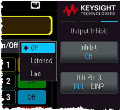
To clear the Inhibit protection function, first remove the external Inhibit signal. Then select **Source Settings > Protection > Protection Clear** for all outputs. This clears the Inhibit protection function and returns the output to its previous operating state.
