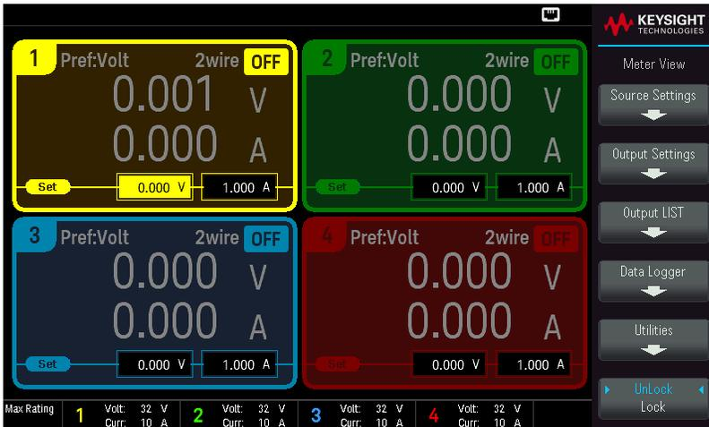
Press one of the four [On] keys to enable an individual output. In meter view, the power supply continuously measures and displays the output voltage and current of each output.
