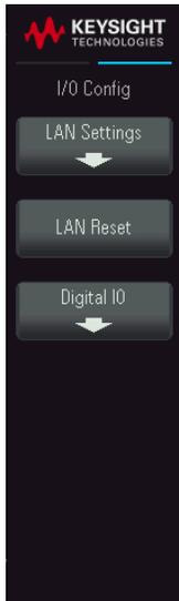
I/O Config displays USB and LAN status as well as configures LAN and digital IO.
