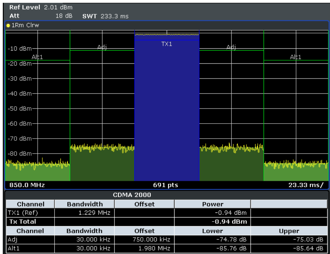
Figure 11-2: Measuring the channel power and adjacent channel power ratio for CDMA2000 1X signals with zero span (Fast ACP)
