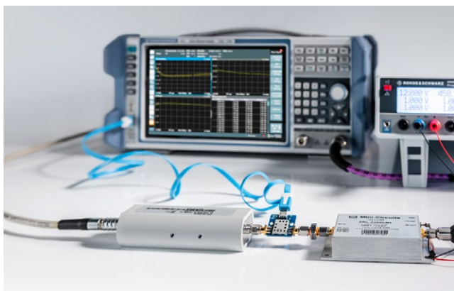
Measuring amplifier noise figure with R&S®ZNL (back), an R&S®FS-SNS18 (left) and an external pre-amplifier (right) powered by an R&S®HMP2030 programmable power supply (back right).
