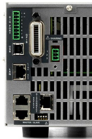
Figure 6. Digital control port on the rear panel
