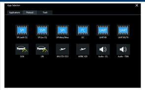
Any protocol can be configured in a few steps from the app cockpit. Once the bus to be decoded and the connected channels have been selected and the levels have been set, decoding begins automatically.
