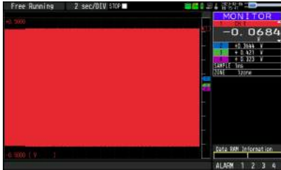
CH1 is active CH. Since the waveform of CH 2 is hidden under the waveform of CH1, it cannot be visually recognized.
