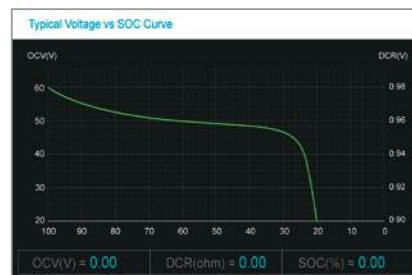
Battery Characteristics V-SOC Curve Setup
