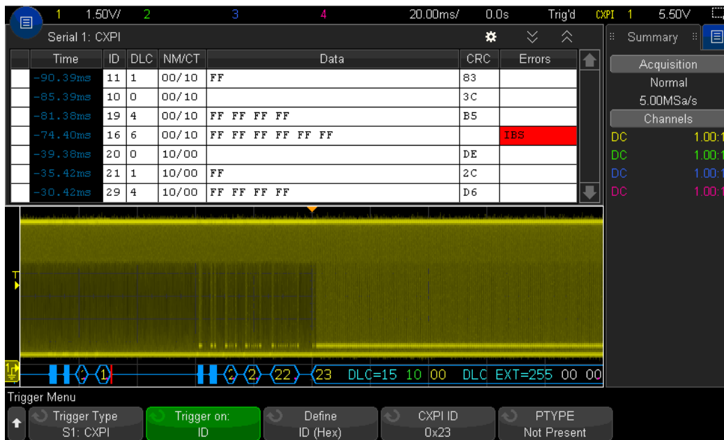
Figure 9. CXPI decode on an InfiniiVision X-Series oscilloscope.
