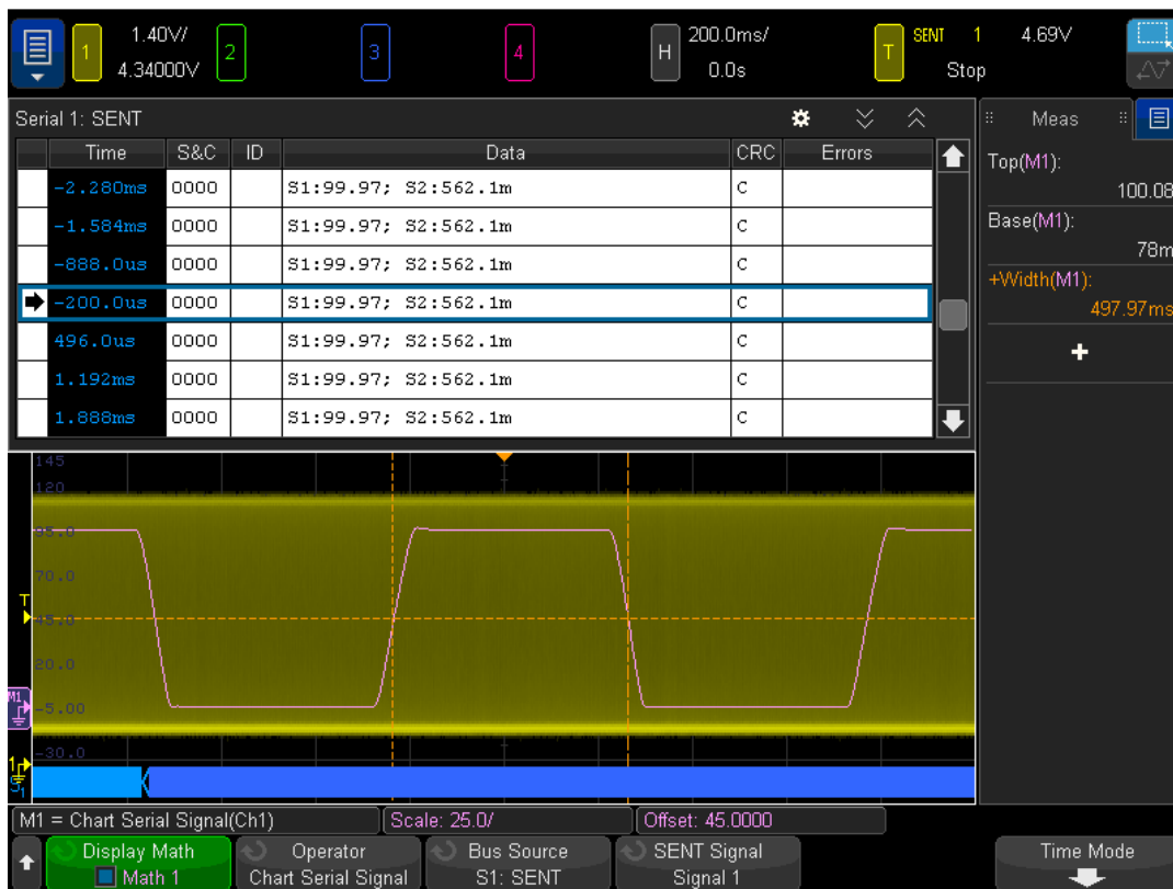
Figure 2. SENT-based throttle blade position signal (S1) charted on the oscilloscope's display.
