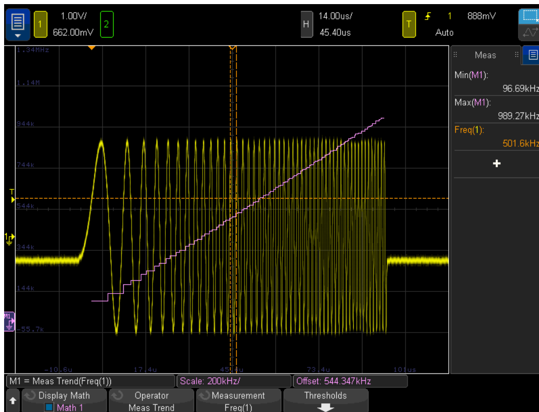
Figure 12. Measurement trend math function used to plot frequency versus time of a FM burst.
