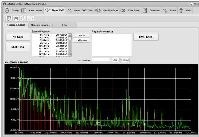
22. Click on the **Pre-Scan** button to start the wide-band measurement. (The setting for this measurement was defined in step 6. When the measurement is finished the spectra graph and a list of peaks are displayed.
