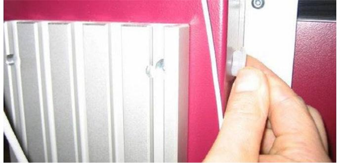
3.18. Lubricate the Z-axis guide shafts using oil.
