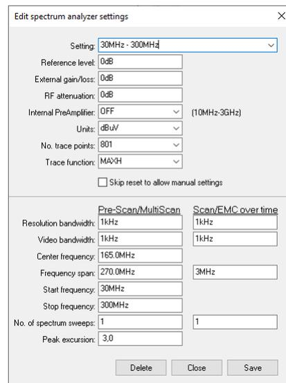
8. Click on the "down arrow" on the right side of the **Setting** box and select a suitable setting from the list showing all stored settings. If no suitable setting is found, you may enter a new setting name and alter the settings.
