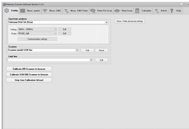
7. In the **Spectrum analyzer** box, near **Setting**, click on the **Edit** button. This is the Settings dialog box.
