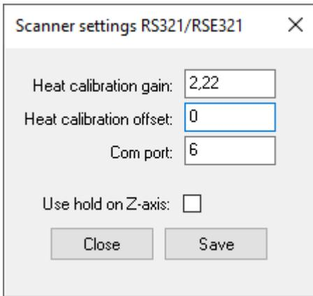
2. Make sure that the **Heat calibration gain** is set to 2.22 and that the **Heat calibration offset** is set to 0 (zero).
