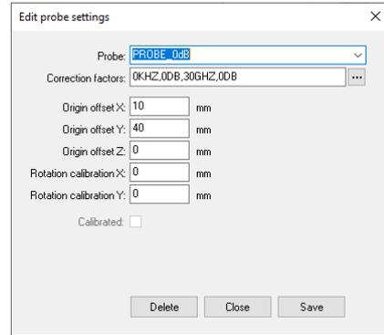
9. Adjust the values of **Origin Offset X and Y** with the distances measured in step 7. For DS, RX and RQ scanners, do not change the value of **Origin Offset Z**. It should always be 10.
