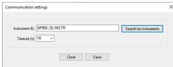
The Search for instruments button will open another dialog that allows for searching for instruments connected id different ways.
