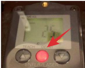
3. Press arrow buttons until the cursor on the display is above the "ε"
