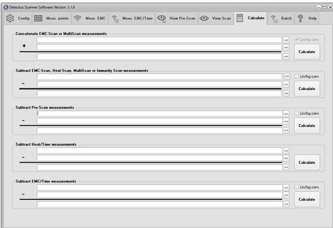
2. **Subtract EMC-Scan or Heat-Scan measurements** is a subtraction, measuring point by measuring point, of two previously saved EMC-Scan or Heat-Scan measurements. This calculation is intended to visualize the difference between two EMC-Scan or two Heat-Scan measurements. For example, one measurement performed before and one after an alteration to the test object.
