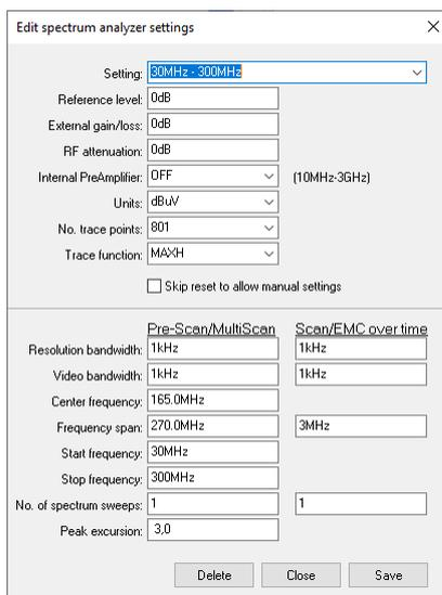
The upper part of the **Edit spectrum analyser** settings dialog box contains settings that are valid for both **Pre-Scan** and **Scan** measurements. In the lower part of the dialog box, the settings for **Pre-Scan** and **Scan** measurements are separated into two columns.
