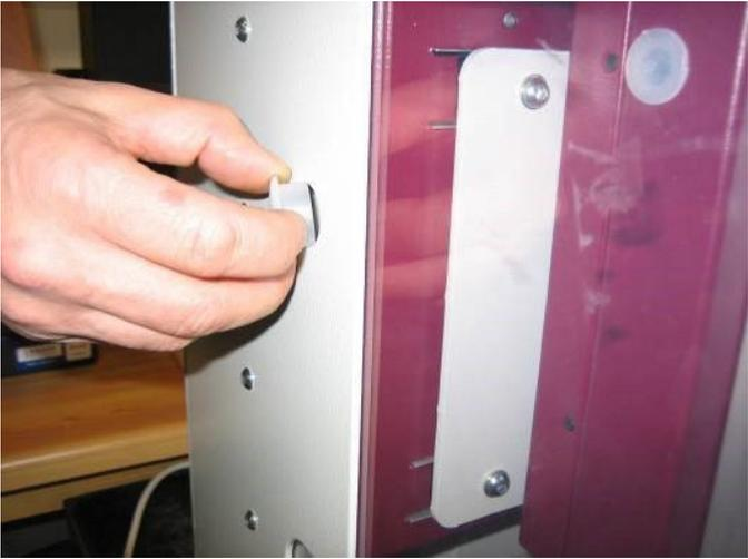
3.11. Lubricate through the now visible nipple using a grease gun.
