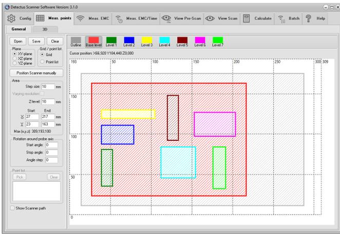
19. Enter a suitable step size in the **Step size** box. A small step size will generate a high-resolution measurement and a large step size will generate a low-resolution measurement. Measuring in large steps is quicker than measuring in small steps.
