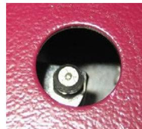
3.9. Lubricate the shaft guides through the sealing lips. Use oil.
