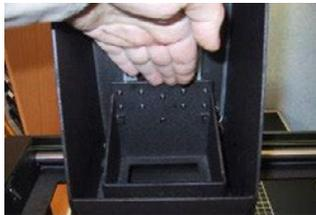
3. Place the probe holder and the probe in the Z-axis carriage (see picture). The probe should point straight down towards the Scanner.
