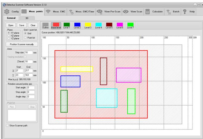
8. Enter a suitable step size into the **Step size** box. A small step size will generate a high-resolution measurement and a large step size will generate a low-resolution measurement. Measuring in large steps is quicker than measuring in small steps.
