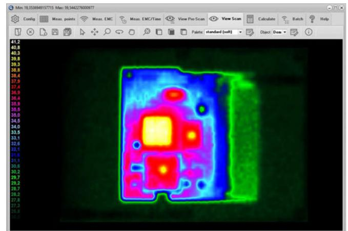
19. There are many ways to visualize the result of a Heat-Scan measurement by utilizing the features on the View Scan tab. For detailed information, please refer to page 131.
