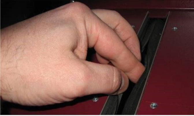
3.10. In order to lubricate the X-axis, push the sledge to the left and remove the plastic plug on the left side of the Scanner.
