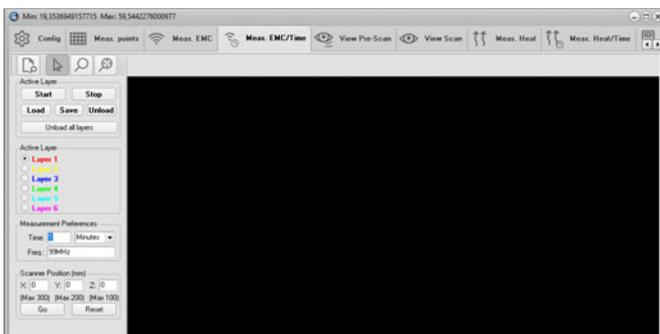
5. Enter the desired coordinates into **Scanner Position (mm)** box, and click on the **Go** button to move the Scanner and place the near field probe above the spot you want to measure.
