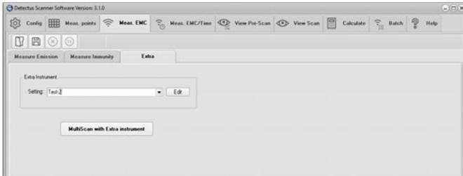
Using the features on this tab you can make MultiScan measurements with an extra instrument performing some task on the side in each measuring position. What this feature can be used for and what type of instrument is up to your imagination. The only requirement is that the instrument must be remotely controllable and Visa compatible.
