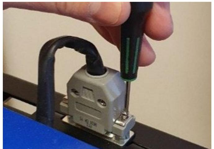
4. Connect the probe holder to the ZR module.
