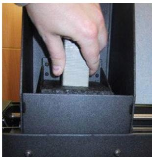
5. Move the Z-axis carriage upwards until the lower limiting position switch is released.
