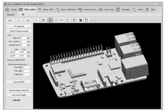
4. Click on the **STL alignment** button. Make sure the 3D model (STL-file) is aligned with the physical object on the scanner table by using the STL-alignment feature described in detail on page 103.
