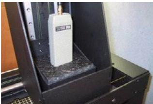
4. Carefully move the probe downwards until the tip of the probe touches the Scanner table.
