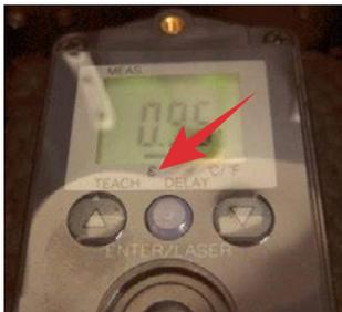
4. Press the enter button to select the emissivity setting mode.
