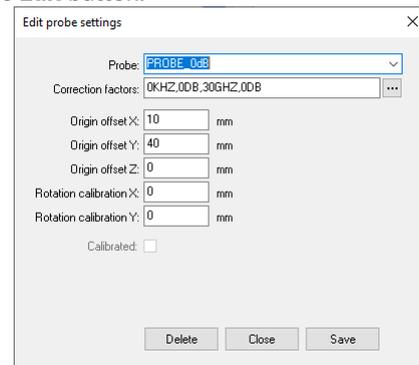
11. Click on the "down arrow" on the right side of the **Probe** box and select a suitable setting from the list showing all stored settings. If no suitable setting is found, you may enter a new setting name and alter the settings to suit you. (Refer to "Entering the amplitude correction factors of the near field probe").
