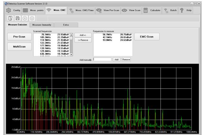
30. Click on the **EMC-Scan** button to start the narrow-band measurement of the selected frequencies. (The setting for this measurement was defined in step 6.)
