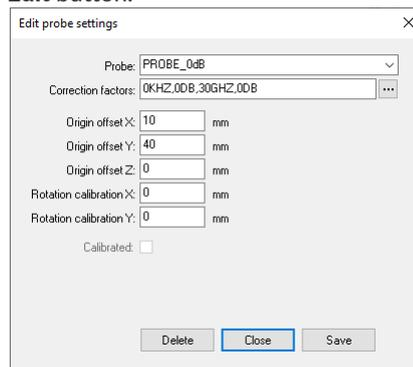
12. Click on the "down arrow" on the right side of the **Probe** box and select a suitable setting from the list showing all stored settings. If no suitable setting is found, you may enter a new setting name and alter the settings. (Refer to "Entering the amplitude correction factors of the near field probe").
