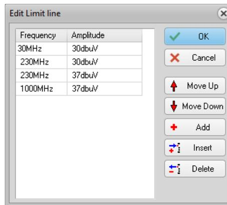
In this dialog box you can add, move, insert or delete frequency values and amplitude values.
