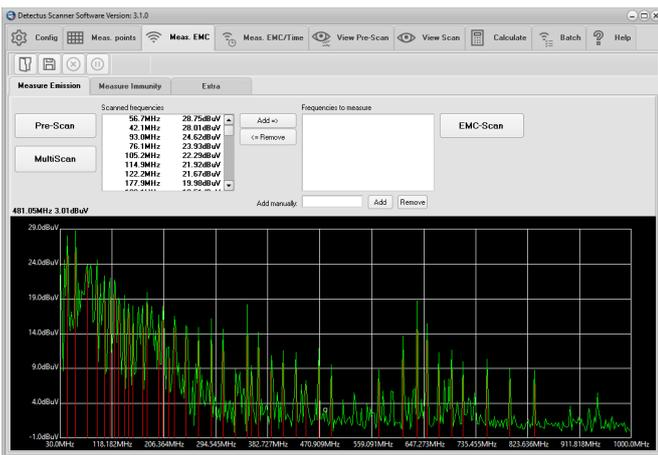
27. Click on the **MultiScan** button to start the wide-band measurement of the selected frequency span. (The setting for this measurement was defined in step 7.) Before the measurement is started, you will have to enter the location to save the result as one or more files.
