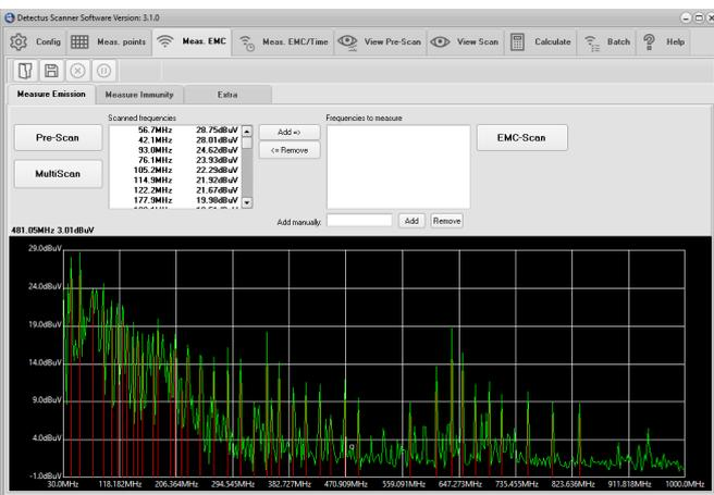
27. Click on the **Pre-Scan** button to start the wide-band measurement. (The setting for this measurement was defined in step 6.)
