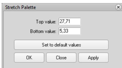
By default, the color palette is set up to cover the total amplitude span of the loaded measurements. By adjusting the top and
