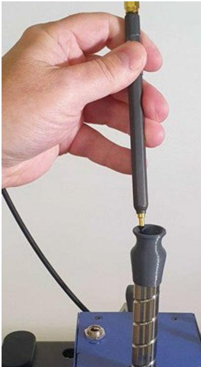
3. Fasten the probe by tightening the nut firmly.
