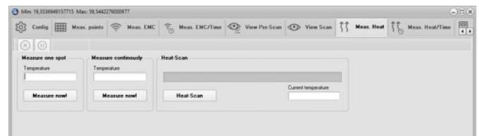
16. Click on the **Heat-Scan** button to start the measurement.
