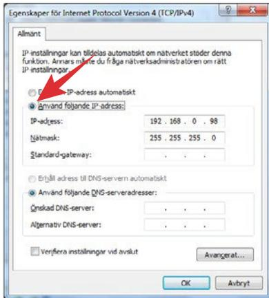
8. Type in IP-address and netmask. The netmask and the three first digit groups of the IP-address should be the same as for the instrument. The last digit group of the IP-address must not be the same as for the instrument.
