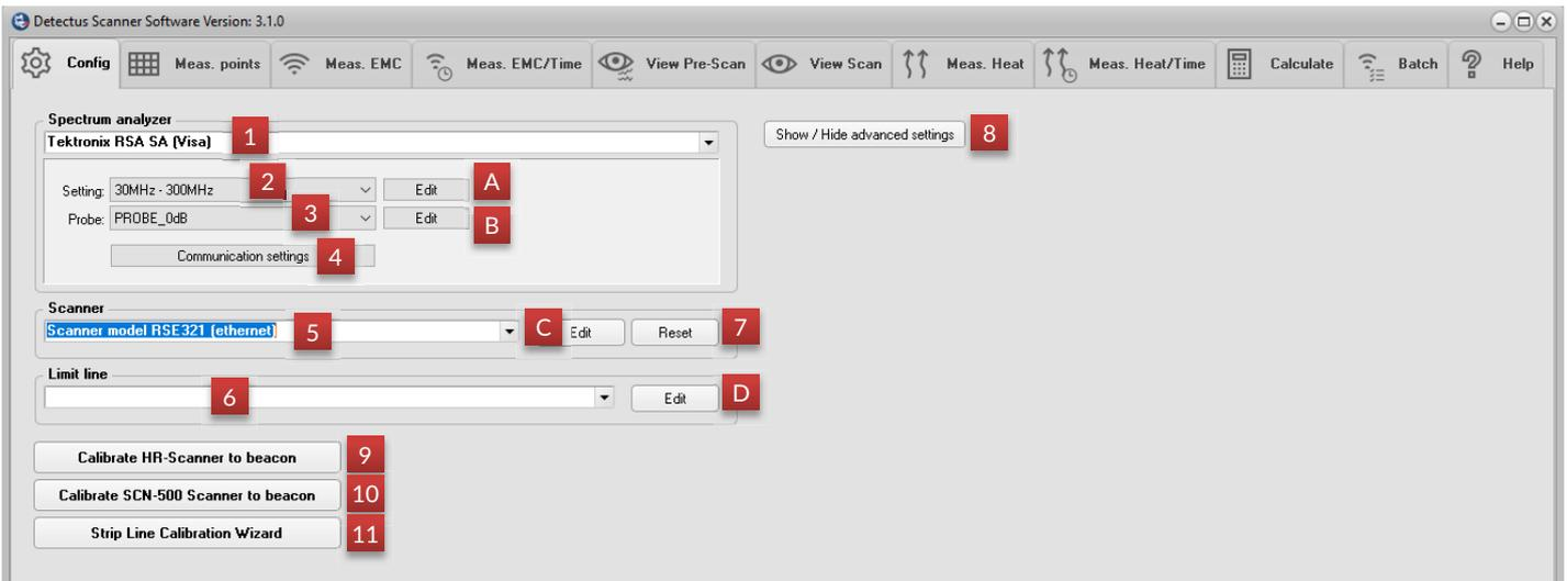
On this tab, you may create your own settings for Scanner, spectrum analyzer, near field probe, IR-probe, limit lines, graphics and reports. You may also use the pre-defined settings.
