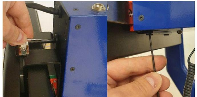
3. Connect the 15-pin D-SUB and secure it with the two screws. Use a regular flat head screwdriver.
