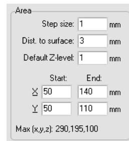
6. Click on the **Generate MP3D** button to generate the measuring points. Generation may take some time if the 3D model is complex. A blue bar will show the progress. Generation can be stopped by clicking again on the same button.
