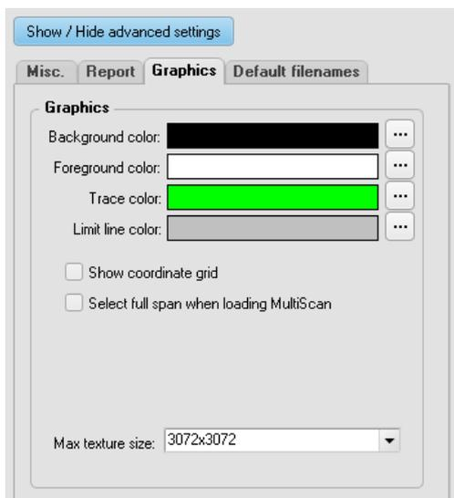
8.3.2 Background color, Foreground color, Trace color and Limit line color: Click on the ... button to select the foreground color of the graphics on the **Measure EMC** tab, the **Measure Heat/Time** tab, the **View Scan** tab and the **View Pre-Scan** tab.
