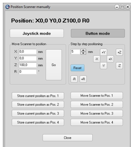
This dialog box will help you move the probe to the preferred position. Use the “Step by step positioning” or “Move Scanner to position” features to move the probe.
