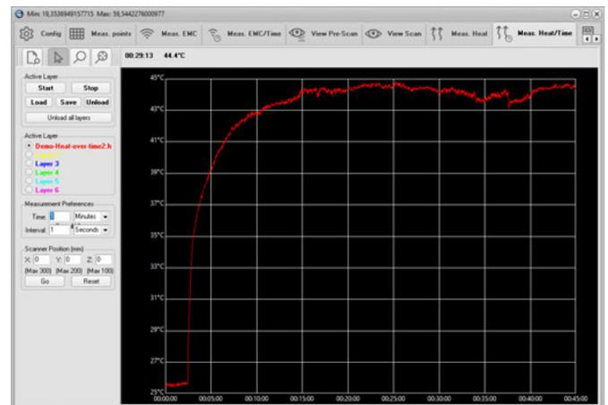
6. Enter the desired coordinates into Scanner Position (mm) box, and click on the **Go** button to move the Scanner and aim the IR-probe towards the spot to be measured.
