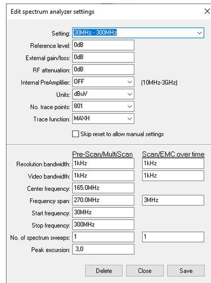
7. Click on the "down arrow" on the right side of the **Setting** box and select a suitable setting from the list showing all stored settings. If no suitable setting is found, you may enter a new setting name and alter the settings.
