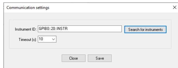
2. Enter the GPIB address of your spectrum analyzer into the **GPIB Address** box.
