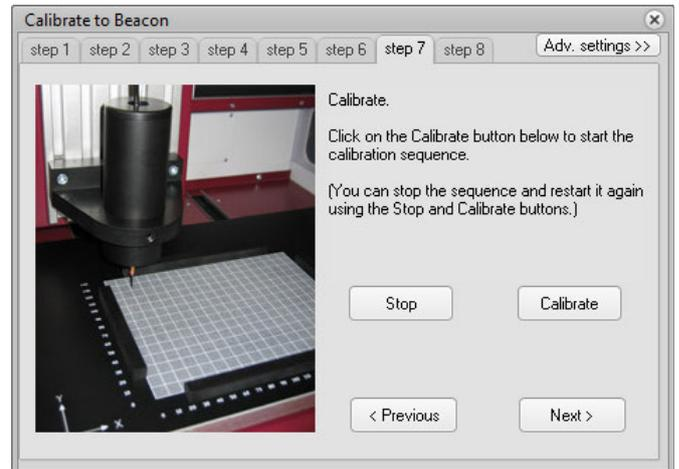
When the calibration is done you will be given a choice to move the probe to XOYOZO. It is recommended to do so. This is a chance to verify that the probe is correctly calibrated. If the calibration was successful, the tip of the probe should be position directly above XOYO.
