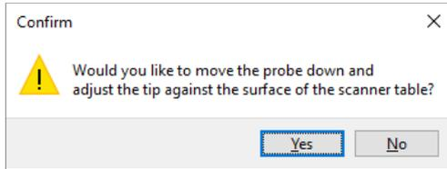
4. Make sure that the probe is mounted high enough, or just remove the probe to be extra safe, before clicking OK to move down.
