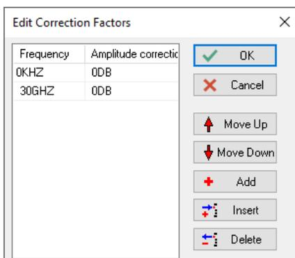
In this dialog box you can add, move, insert or delete frequency values and amplitude values.
