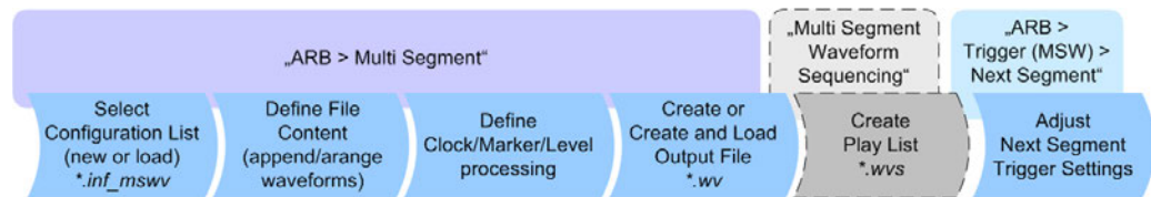
Figure 4-27: Basic workflow for generation of multi-segment waveforms
