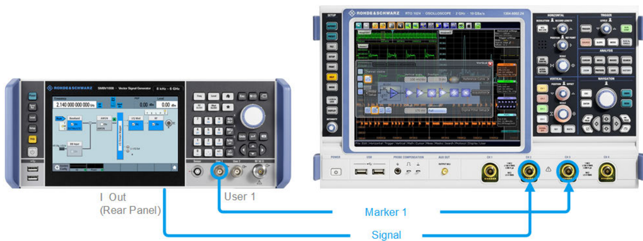
Figure 3-11: Simplified representation of a test setup for signal monitoring**
