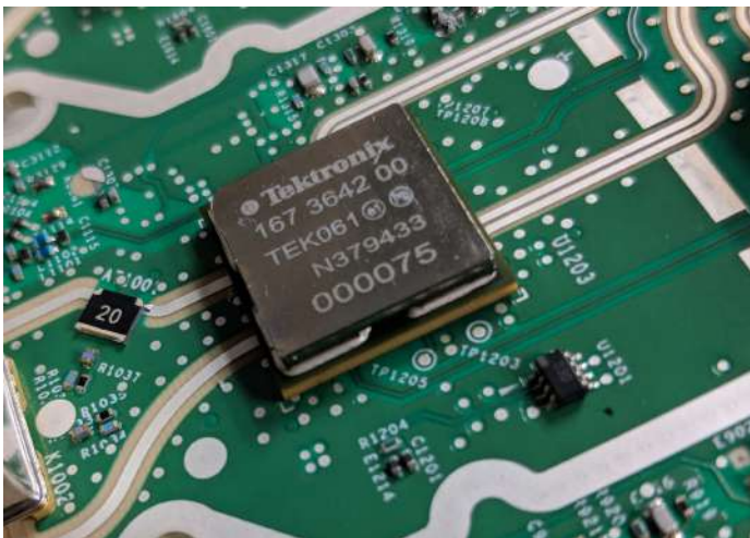
A new TEK061 front end amplifier sets a new standard for low-noise acquisition providing the best signal fidelity to capture small signals with high resolution.
