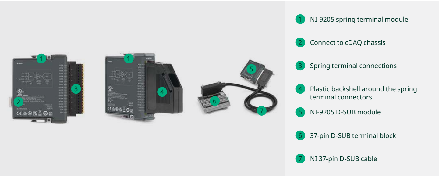
FIGURE 2 Several modules are available with different connectivity options, such as the NI-9205.
