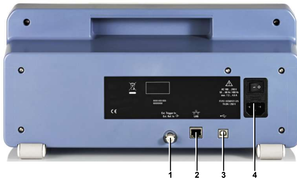
Figure 3-2: Rear panel of the R&S FPC
