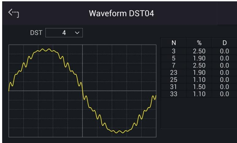
In Meas. & Setup (3\_Phase Mode/1\_Phase Mode) main page, set the Vac to 100.0V and then tap **ON/OFF** to enable the waveform.
