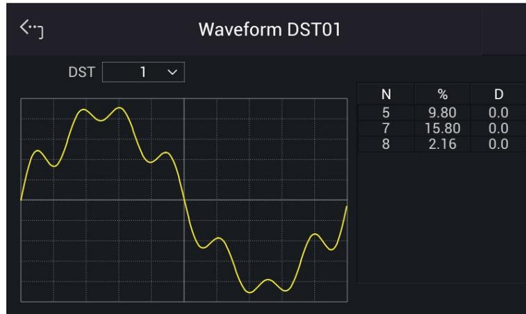
Follow the steps below to set the 3-phase waveform to clipped sine with a total harmonic distortion of 35%.
