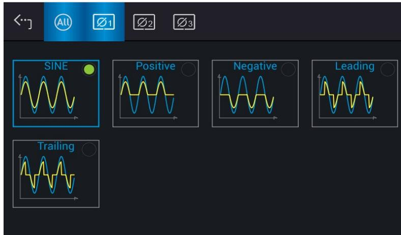
Set the 3-phase waveform to Leading-edge wave at the same time:
