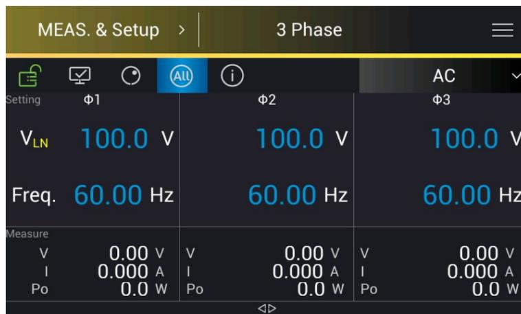
2. When AC+DC is selected for coupling output mode, the output voltage will be restricted by voltage specification.
