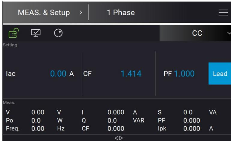
When set to Lead, it means that the current loading phase leads the UUT voltage phase. When set to Lag, it means the current loading phase lags behind the UUT voltage phase.
