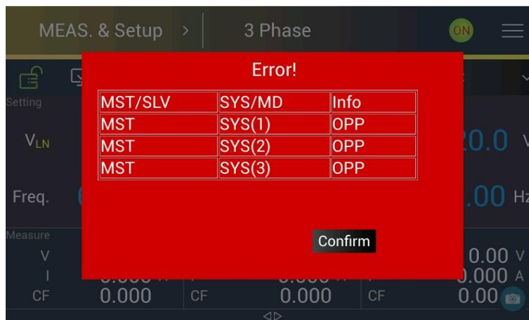
If unable to determine the cause of the error it is recommended to remove the load and restart the Regenerative Grid Simulator to release protection for normal operation.
