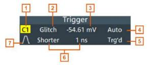
Figure 6-2: Trigger label on the toolbar
