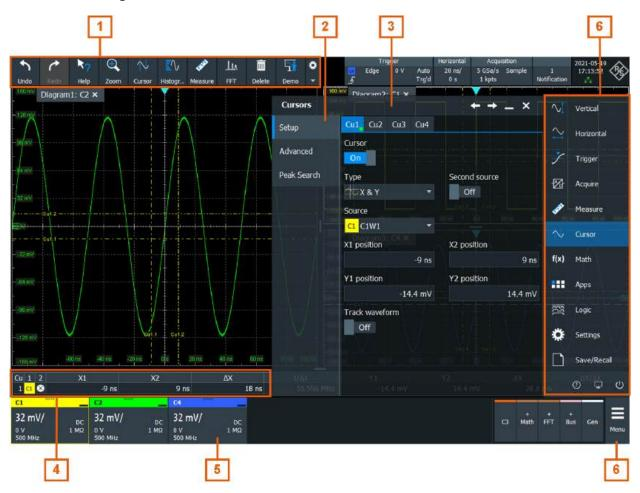
Figure 6-6: Control elements on the touchscreen
