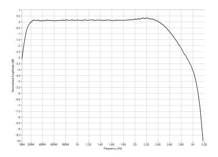
Figure 6. Analog Output Single Channel Mode Frequency Response With Anti-Image Filter, Measured<sup>14</sup>
