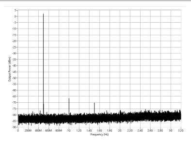
Figure 2. Single Tone Spectrum (Dual Channel Mode, 1.01 GHz 0 dBFS), Measured<sup>11</sup>
