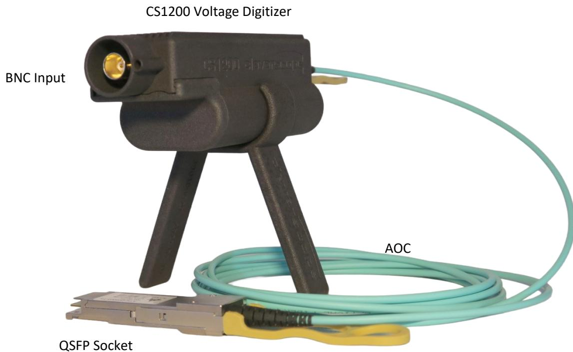
The CS1200 allows time aligned measurements to be made between locations up to 60m apart (using 30 m cables), and measurements in hazardous, high voltage situations. The VD batteries are standard 21700 5AHR cells and offer more than 6 hours operation before recharge. One set of cells can be recharged while the other set is being used. Cleverscope supplies two sets of batteries, and a charger.
