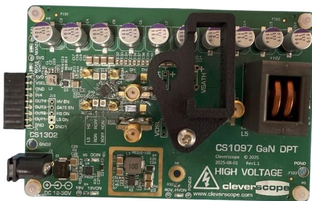
Demo board is equipped with 3x CS1501 current shunts for use with CS1201 for testing source currents on High- & Low-Side (one each) and for inductance load current.
