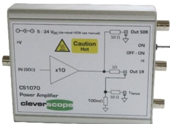
It has 50 MHz BW, and can swing  $\pm 17$  V, and can be offset up to a maximum of 32 V. The 50R output is useful for driving impedance matched coaxial cables, while the 1R output can drive low impedance loads such as power and ground planes and power supplies. If battery driven it can be isolated using the CS548 isolated signal generator.
