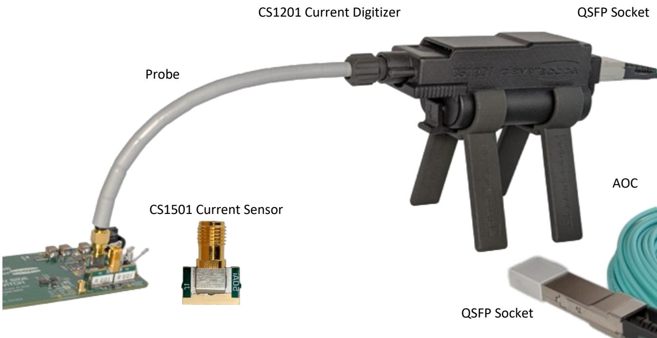
The CS1201 allow time aligned measurements to be made between locations up to 60 m apart (using 30 m cables), and measurements in hazardous, high voltage situations. The CD batteries are standard 21700 5 AHR cells and offer more than 6 hours operation before recharge. One set of cells can be recharged while the other set is being used. Cleverscope supplies two sets of batteries, and a charger.
