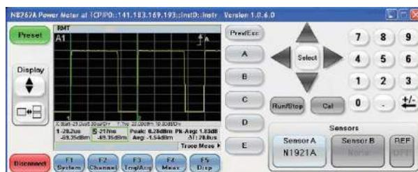
Control an N8262A and view measurement results through the Power Meter GUI soft front panel, the way you would a P-Series power meter from its front panel.
