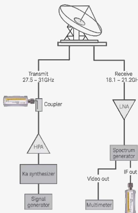
Typical satellite test system set-up
