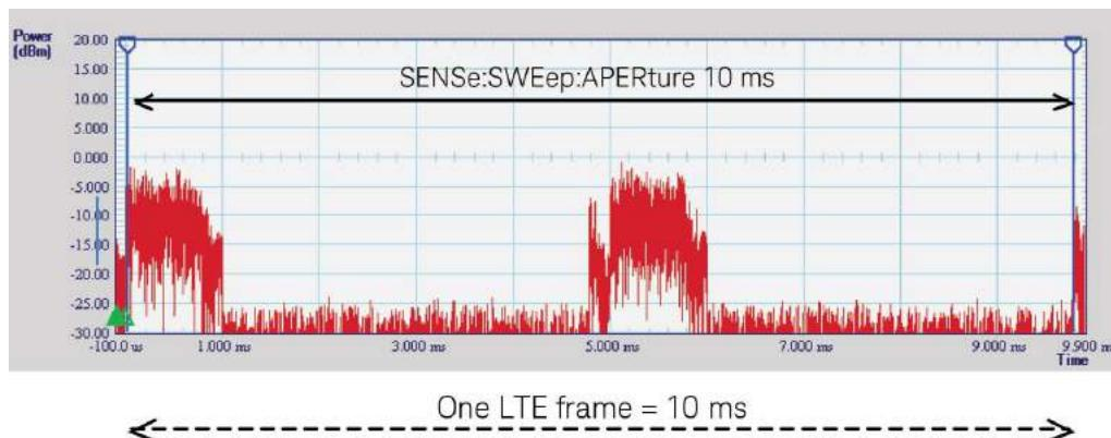
Measurement of one LTE frame over 10 ms using waveform average power setting.
