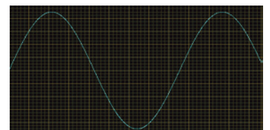
Filter On: Bandwidth = 5kHz (meets the 3kHz requirement of Energy Star)
