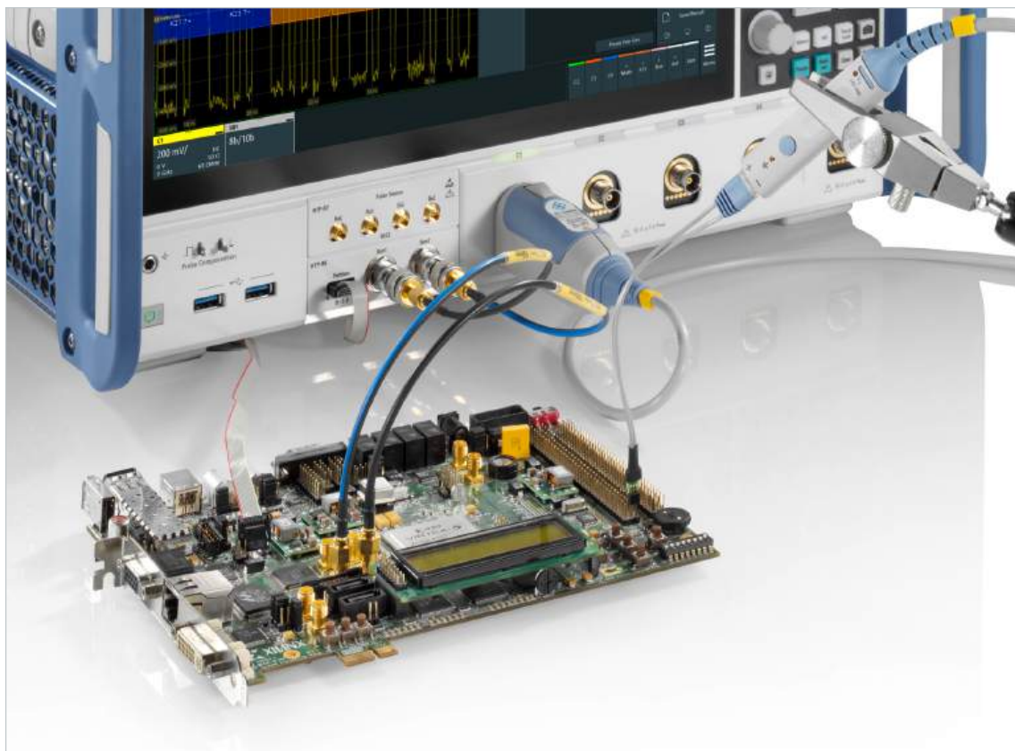
Measurement of LVDS signals using the integrated arbitrary waveform generator as the clock signal and the 8 bit pattern generator to program and control the device
