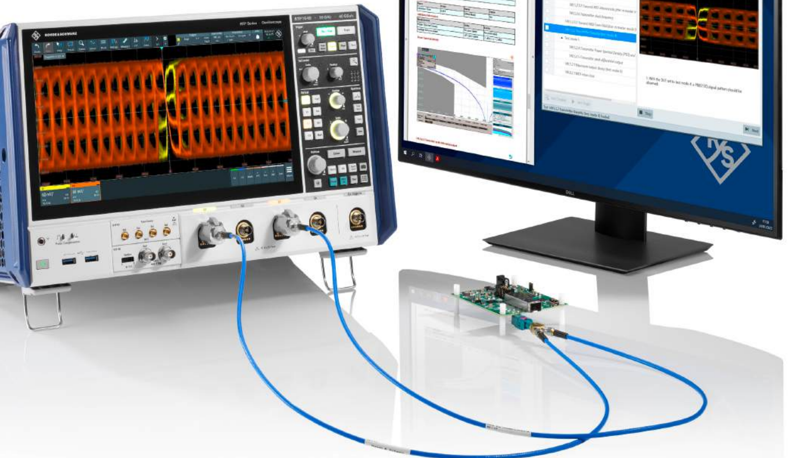
Automated Auto Ethernet compliance test
