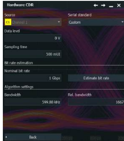
The configurable HW-CDR of the R&S®RTP supports data rates up to 16 Gbit/s for data eye analysis.
