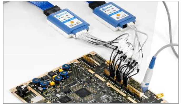
Every R&S®RTP can be upgraded on site with 16 digital channels
