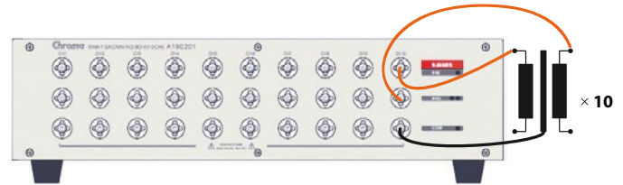
Figure 8 : A190201 with 3 way scanning
