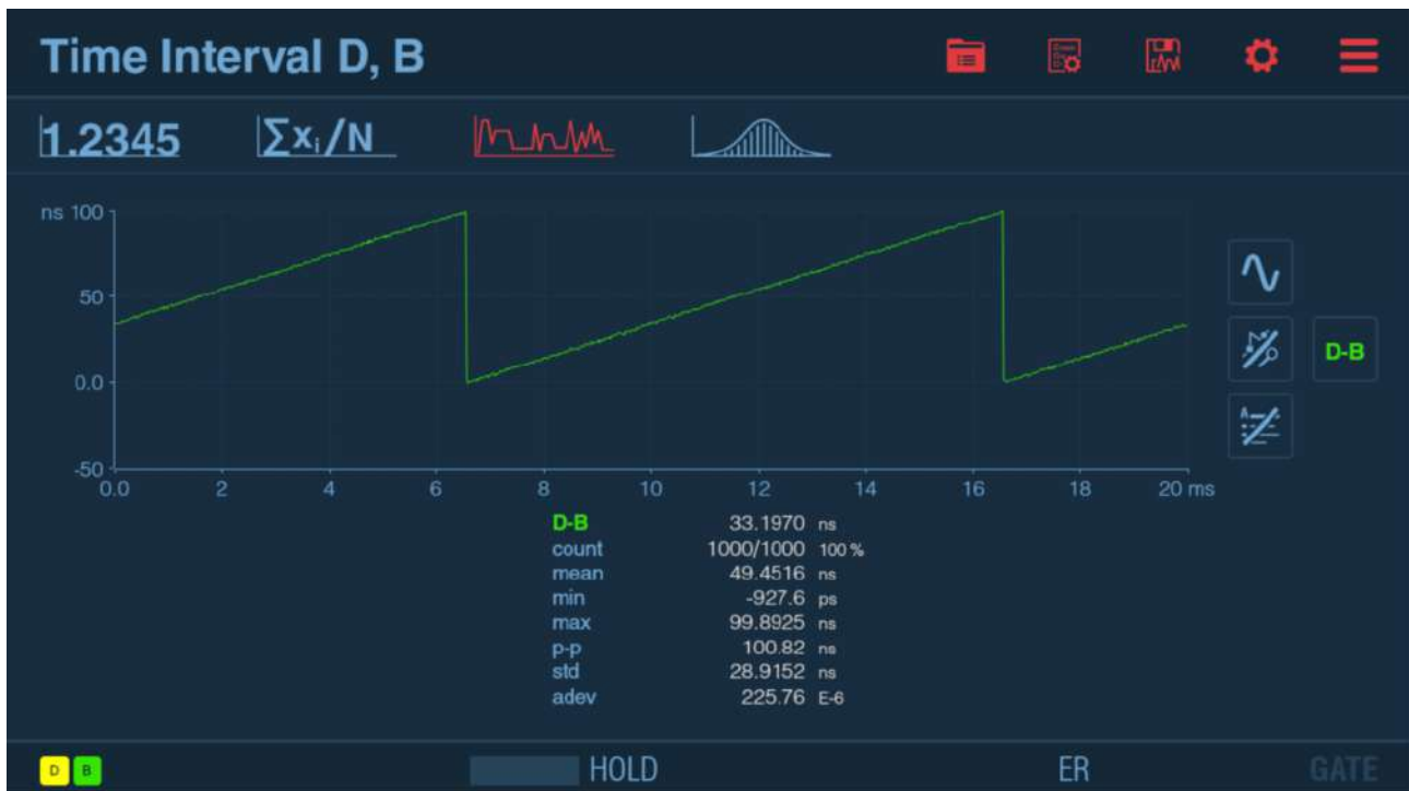
Fig. 5.8: Time Interval Continuous of 2 clock signals with constant frequency offset
