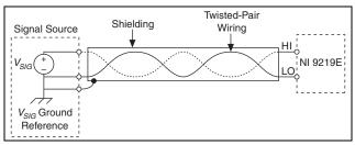
Figure 4. Connecting a Grounded Signal Source to the NI 9219E
