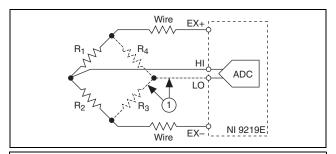
1 The dotted line represents the portion of the circuit that is connected only in Full-Bridge mode.
