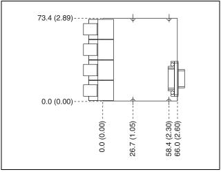
Figure 1. NI 9219E Dimensions in Millimeters (Inches)
