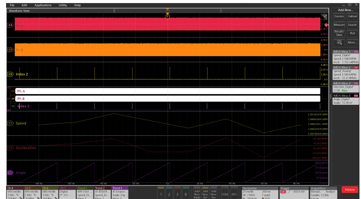
Measuring motor speed and direction using QE1 method. The QE1 signals (Phase A, B, and Z index) are shown for reference by connecting both Analog (TPP1000) and Digital (TLP058) probes.
