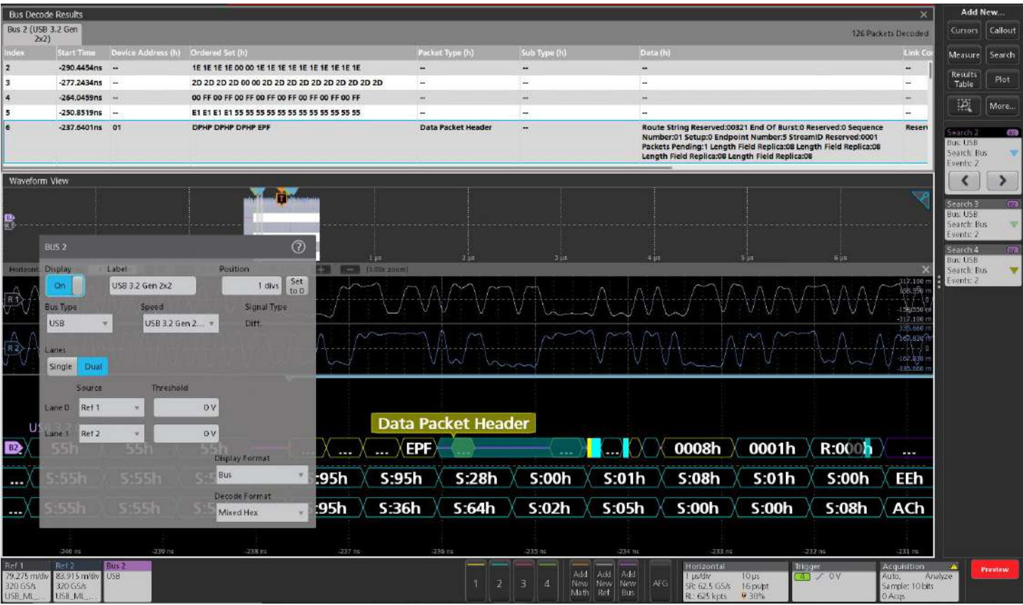
Bus configuration for the USB bus with decode speed USB 3.2 Gen2x2 for the DP packets. Search on packet type LMP along with lane 0 and lane 1 search on training sequence is added.
