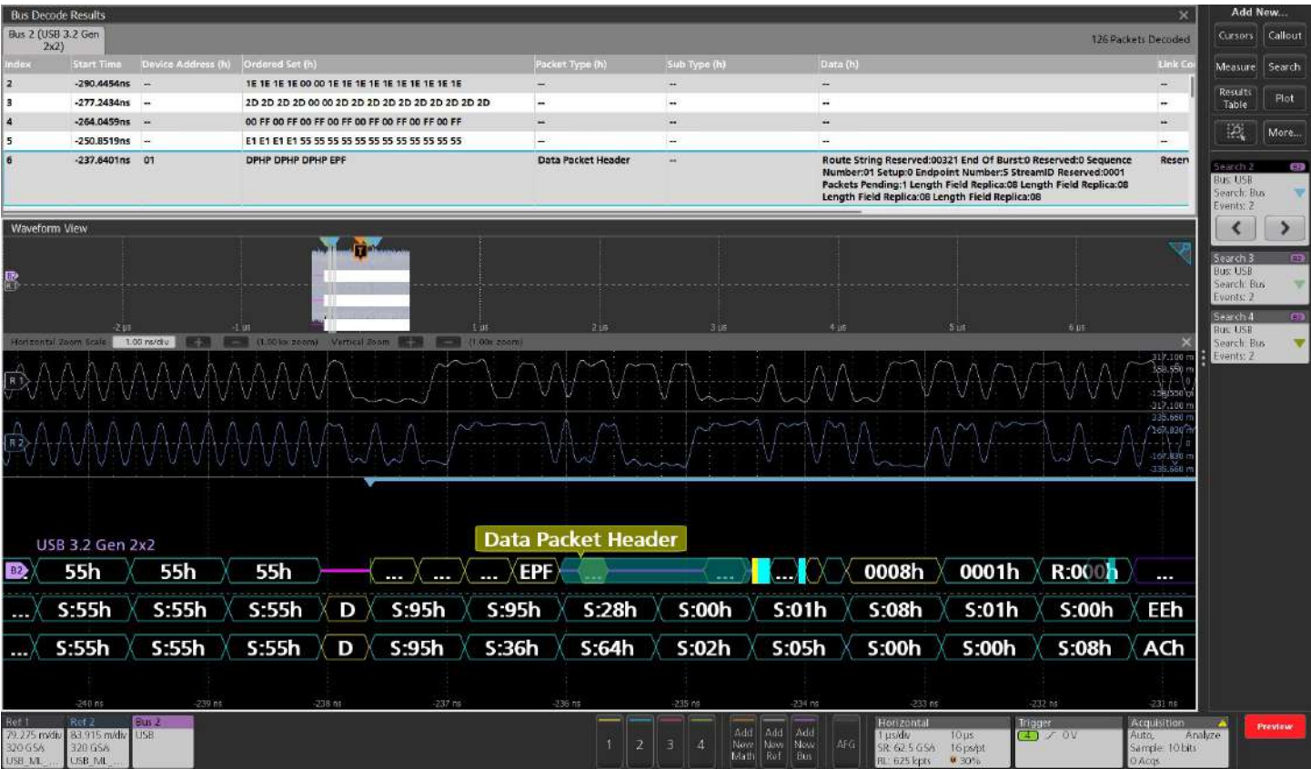
Searching the USB bus with decode speed USB 3.2 Gen2x2 for the DP packets. The results table at the top of the graticule.
