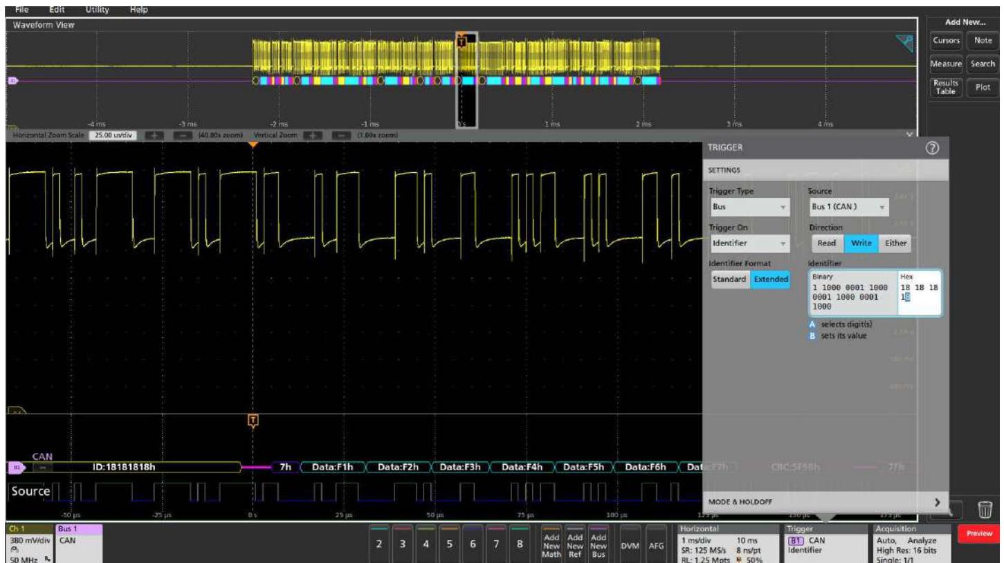
Triggering on a specific extended Identifier value on the CAN bus.
