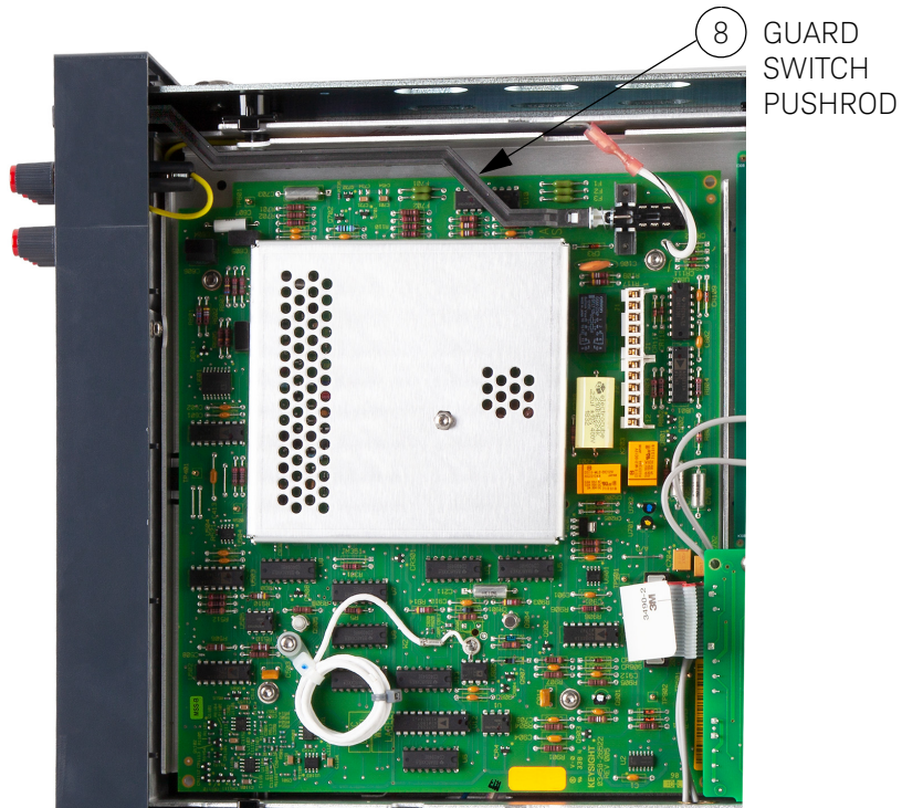
Figure C-6 Guard switch and pushrod location
