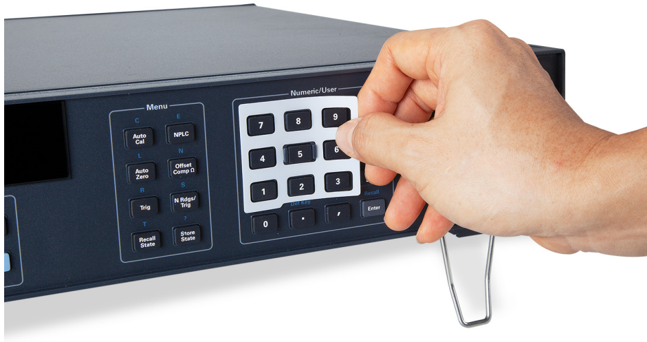
Figure 2-7 Installing the keyboard overlay
