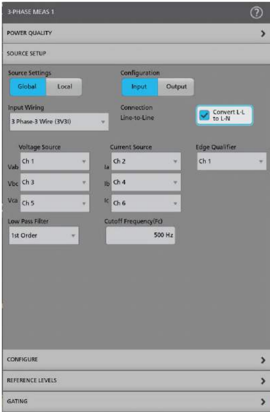
Figure 4: Configure Power quality measurement as Input or Output. Optionally convert Line-Line to Line-Neutral configuration mathematically without physical connection changes.
