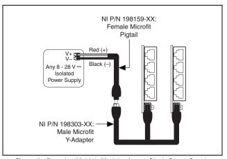
Figure 4. Powering Multiple Modules from a Single Power Supply
