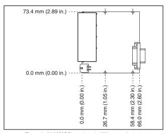
Figure 1. NI 9870E Dimensions in Millimeters (Inches)
