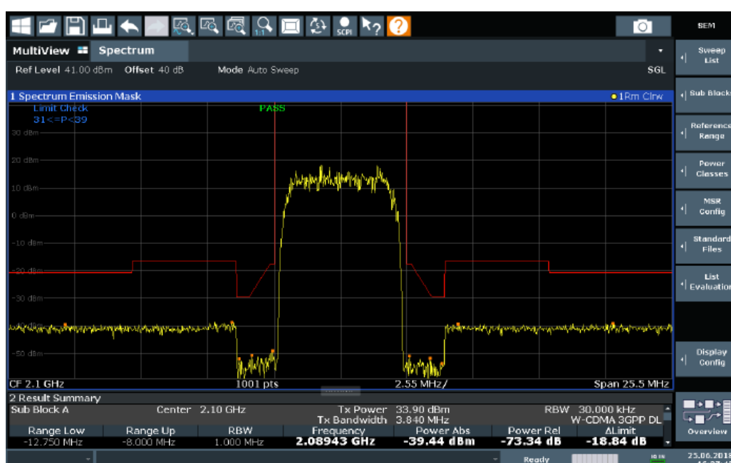
Figure 6-26: Detected peak display in SEM measurement
