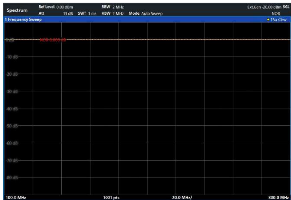
Figure 6-48: Normalized measurement results after calibration
