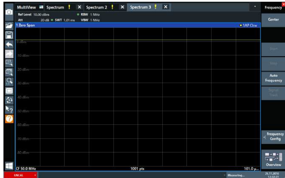
Figure 4-10: Time domain display of the calibration signal
