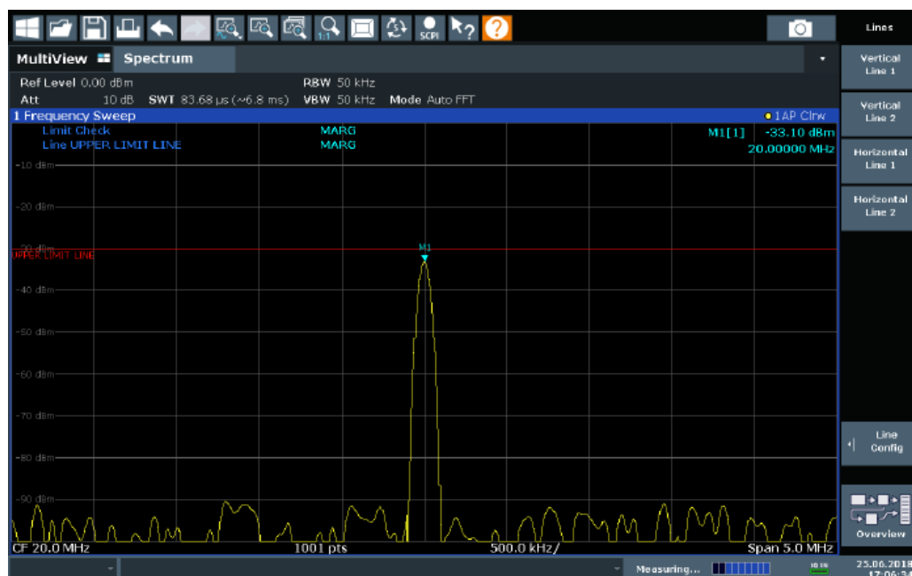
Figure 6-78: Margin violation for limit check
