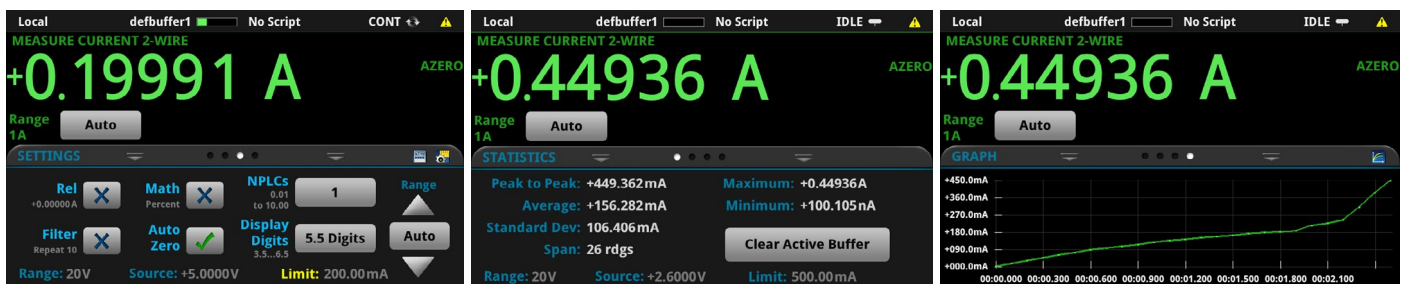
Figure 10: Three various swipe screen views on the secondary information line of the 2460/2461.
