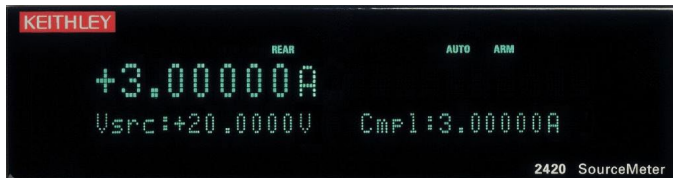
Figure 8: Display contents of the 2420 SMU
