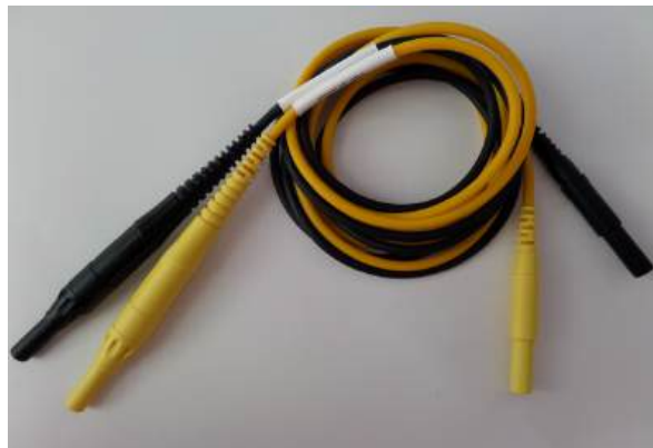
Figure 5.18: Fused safety laboratory leads for voltage path
