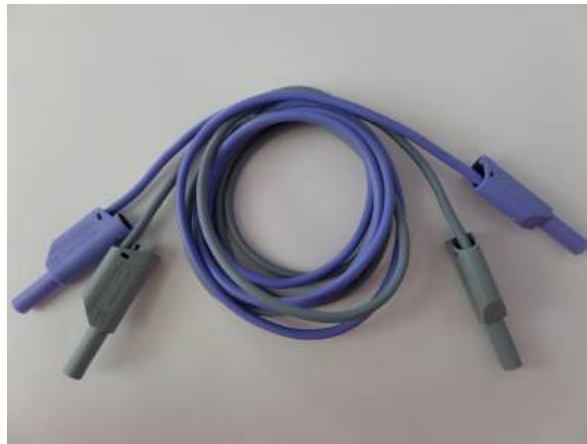
Figure 5.17: Safety laboratory leads for current path
