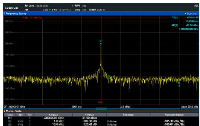
Simple phase noise measurement with a marker function
