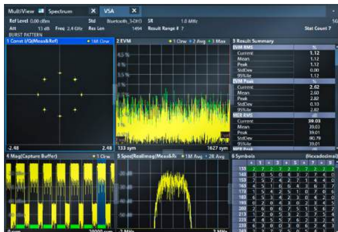
Demodulation of a Bluetooth® signal with the R&S®FPL1-K70 option
