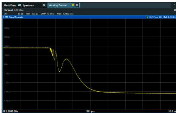
Frequency settling behavior of an oscillator
