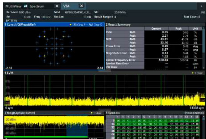
Demodulation of a DVB-S2 multi-modulation signal with the R&S®FPL1-K70M option (R&S®FPL1-K70 option required)
