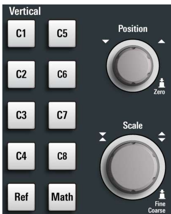
Figure 5-5: Vertical controls of MXO 5 with 8 input channels
