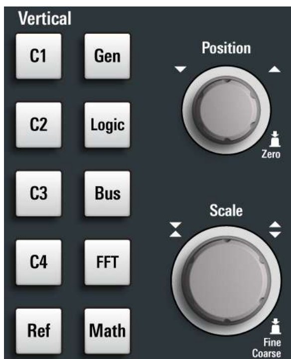
Figure 5-4: Vertical controls of MXO 5 with 4 input channels
