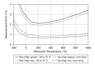
Figure 5. Thermocouple Type B Errors
