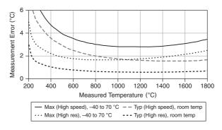
Figure 6. Thermocouple Types R and S Errors
