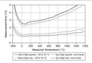
Figure 4. Thermocouple Types T and E Errors
