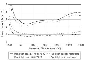
Figure 3. Thermocouple Type K Errors
