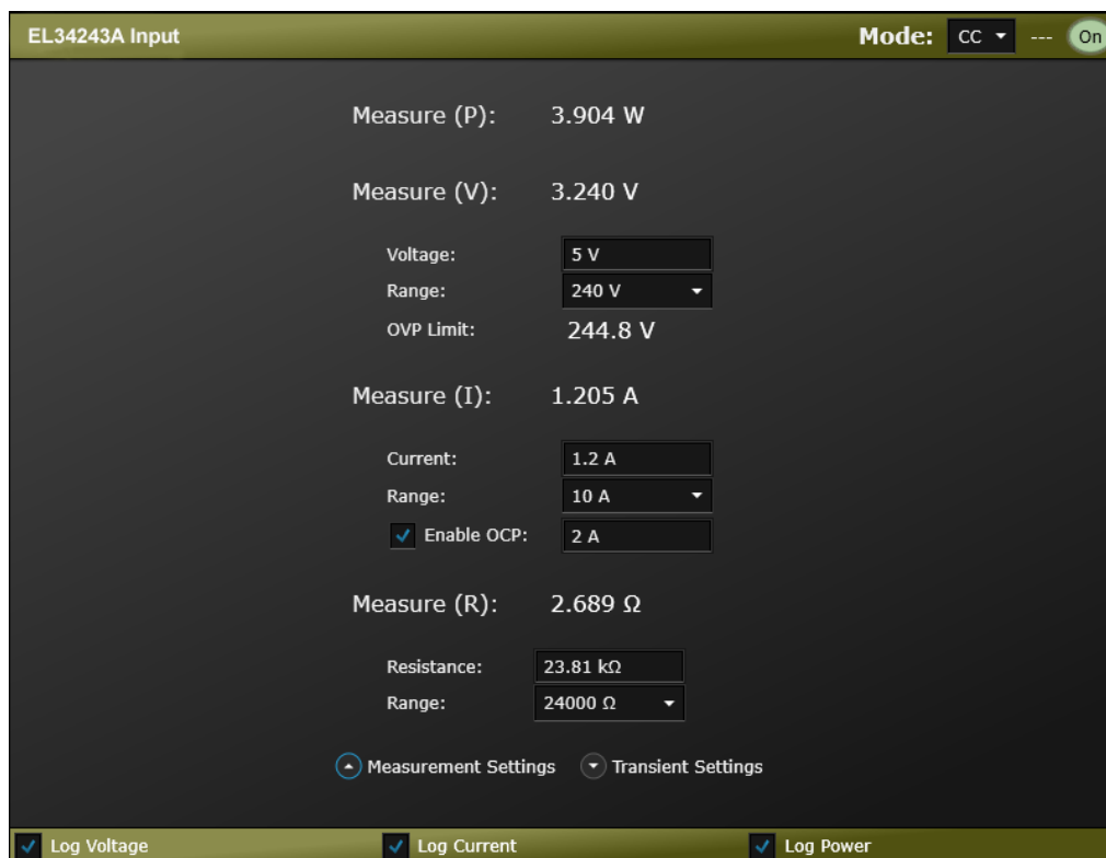
Figure 6. BenchVue Electronic Load app configuration.
