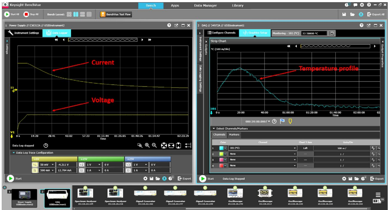
Figure 7. Temperature, voltage and current profiles shown in strip chart format on the BenchVue software while battery is charging.
