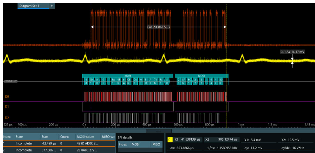
Figure 13-3: Decoded and binary SPI signal
