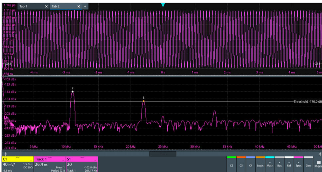
Figure 9-8: Track and spectrum on track, C1 is not in diagram
