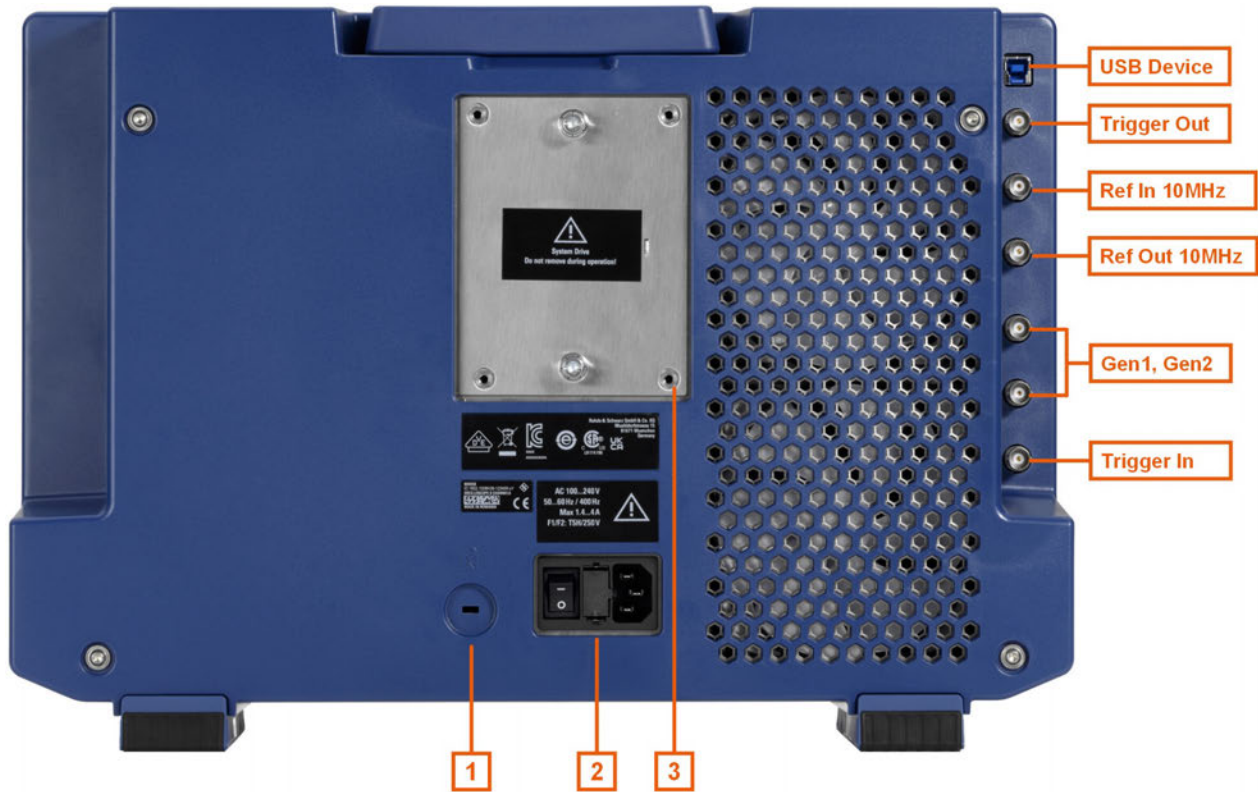
Figure 3-3: Rear panel view of R&S MXO 5
