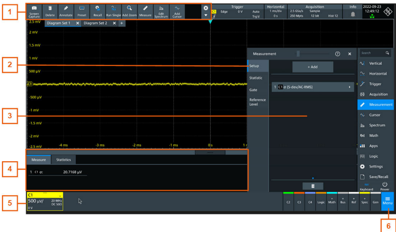
Figure 4-6: Control elements on the graphical user interface
