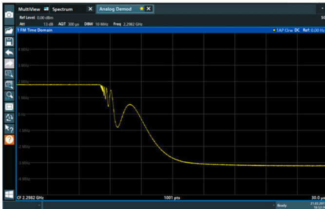
Frequency settling behavior of an oscillator
