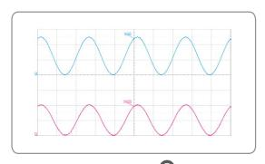
CT-PCB Voltage Output – "V" Version  $C_{LUCS}$  DC + 20-kHz sine-wave primary current – i.e.  $I_p$  [A] – and output voltage of a CT-13V version – i.e.  $V_o$  [V]
