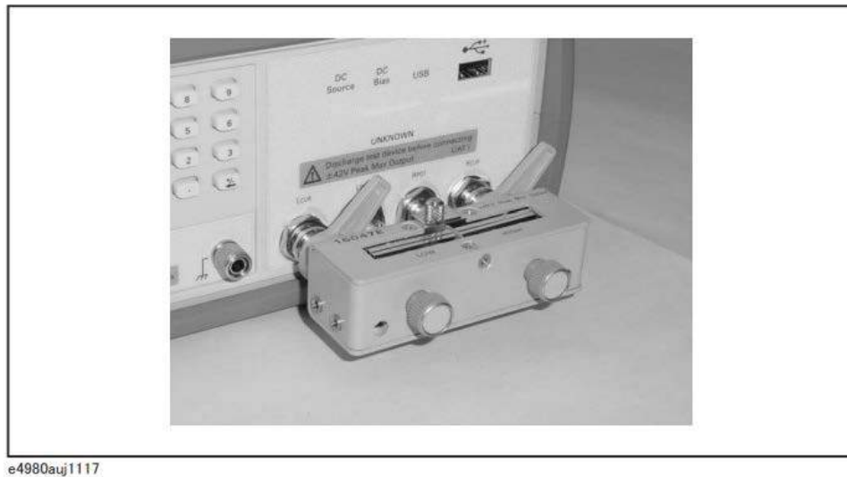
Figure 7-18 Connecting the 16047E
