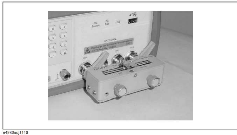
Figure 7-19 Connecting a shorting bar
